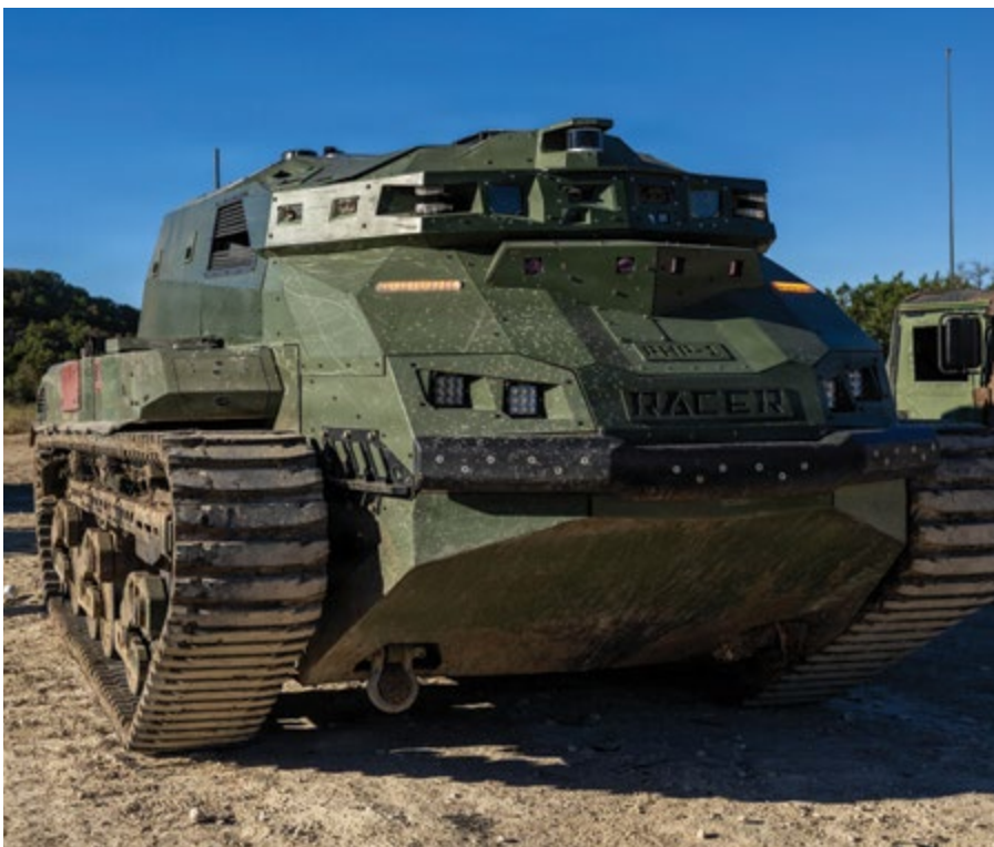
Figure 4. RACER technologies that enable Unmanned Ground Vehicles (UGVs) to maneuver on unstructured, off-road terrain at speeds that are only limited by considerations of sensor performance, mechanical constraints, and safety. (Photo by Thomas Sakell)
